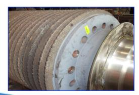
The Perforated / Lotus roller was designed primarily to be used as the top roller in any 3-roller mill; it is also advantageous as the discharge roller of the last mill. As with the Lotus Roller, the Cast Iron / Steel shell has radial perforations leading to axial channels in its body; drainage of juice from the axial channels and thus enhancing the advantages of the Lotus roller as following,
